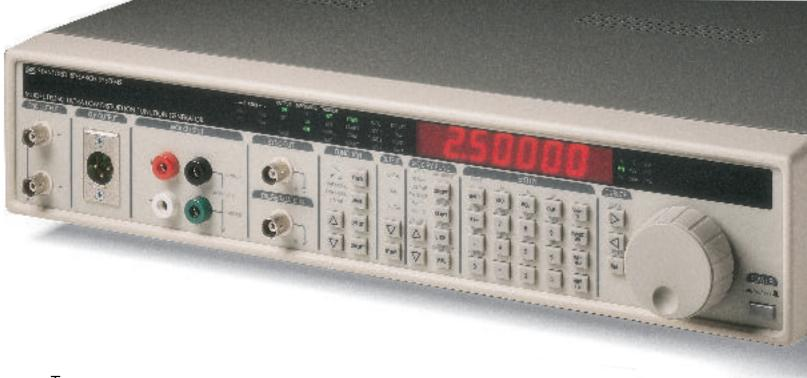
The performance of a low distortion analog source and the precision of direct digital synthesis (DDS) is combined in a unique new instrument - the DS360 from SRS. With less than 0.001% total harmonic distortion (THD), 25 ppm frequency accuracy and a broad range of features including standard waveforms, sweeps and bursts, the DS360 is the ideal source for audio frequency applications.
